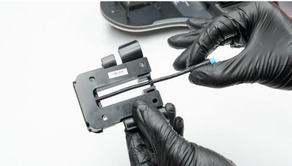
\*\*NOTE\*\* Boosted Mini (shortboard) risers are not interchangeable with longboard risers. The risers are labeled to help ensure you are using the designated rear riser for the correct board.
