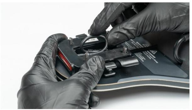
5. Use a skate tool to reinstall your rear truck. Allow the excess cable to sit in the opening on the board side of the truck's baseplate. Be careful to avoid pinching any wires.
