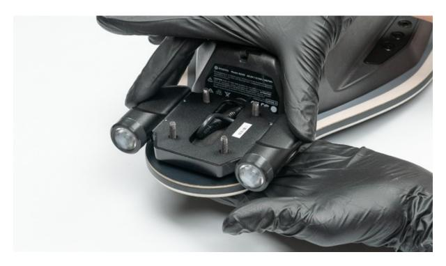
5. Reinstall the front truck using the skate tool. Let any excess cable rest in the channel on the board side of your truck's baseplate. Be careful to avoid pinching any wires.
