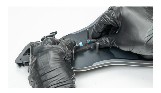
4. Mount the brake light and riser onto the board. The brake light cable should make a loop in the opening located in the middle of the brake light.
