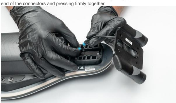
4. Use your finger to guide the headlight cable into the channel on the riser, then seat the headlights over the mounting screws.
