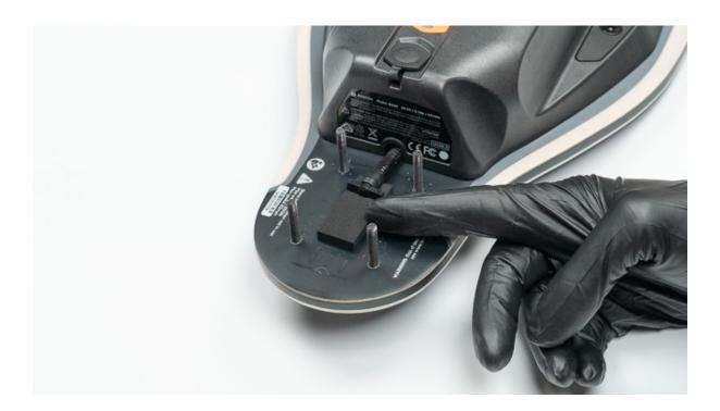
2. Remove the front accessory port cap and install the designated front riser.
