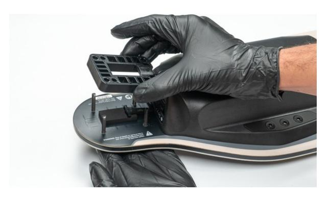
\*\*NOTE\*\* Do not remove the foam pad underneath the accessory port.
