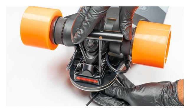
6. Clip your motor cables into the cable clips on your rear riser.
